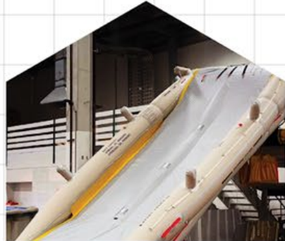
2. Sill Height Testing Deployment
